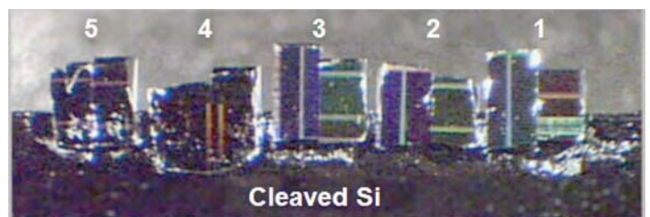
The specimens are affixed in pairs and mounted using hot wax to a cleaved rectangular Si carrier bar.
