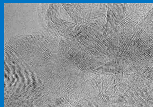
C-lattice fringes, showing 0.34nm resolution, typical for all Gatan cooling holders
